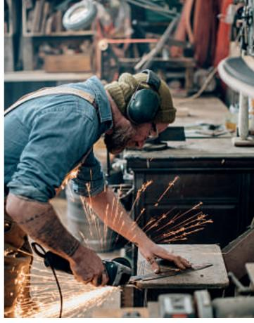
**ABOVE** Reclaimed timber cut-offs that will become handles. ABOVE RIGHT A knife is rough grinded into shape and then heat treated and quenched, before grinding again. RIGHT "The heat treatment and quenching is what hardens it all up and turns it into knife steel," explains Sam. BELOW Blades awaiting handles. "There are two types of handle," according to Sam. "A Western-style of two pieces riveted together or a Japanese style, in which the knife slots into the handle."
